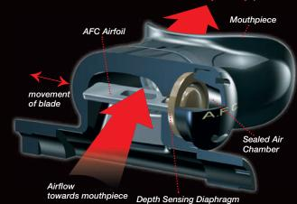
Atomic Aquatics has developed the first and only automatic flow control that automatically changes the breathing characteristics with depth. At depth, the air density increases (gets thicker) and it becomes harder to move through the regulator. The result is increased breathing effort at depth. Many regulators have different types of devices to increase flow (venturi) but these are either fixed in place or manually set and
