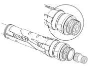
(3) Refit the hose and tighten the ball nut on to the second stage using 11/16" spanner to hold the heat exchanger. Tighten if possible, using an 11/16" crowfoot torque wrench to 5Nm.
