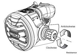
This adjustment is particularly useful at deeper depths, or in variable conditions that affect the opening effort of the second stage, such as strong currents or while using a diver propulsion vehicle (DPV). You can use the inhalation control knob to tune your regulator to maintain its peak performance throughout the course of your dive, or you can leave it set in its mid-range position and dive with it as you would any non-adjustable second stage.
