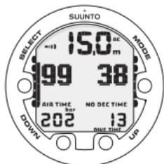
The change in your air consumption is based on constant one second interval pressure measurements over 30–60 second periods. An increase in air consumption influences the remaining air time rapidly, while a drop in air consumption increases the air time slowly. In this way, an over optimistic air time estimation, caused by a temporary drop in air consumption, is avoided.
