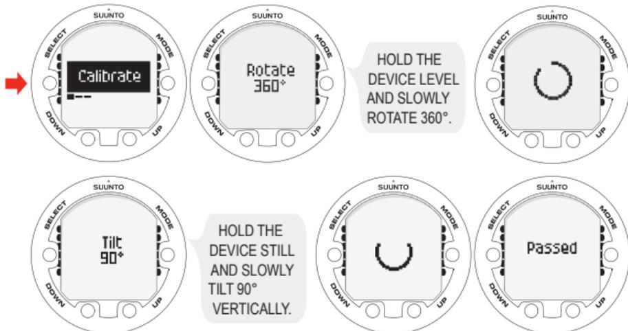
If the calibration fails several times in a row, it is possible that you are in an area with sources of magnetism, such as large metal objects, power lines or electric appliances. Move to another location and try to calibrate the compass again. If the calibration continues to fail, contact an authorized Suunto service center.
