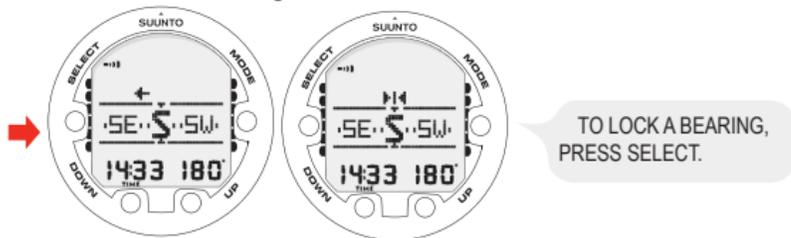
The Suunto Vyper Air also provides help for navigating square and triangular patterns, as well as navigating a return heading. This is made possible by following graphical symbols in the center of the compass display:
