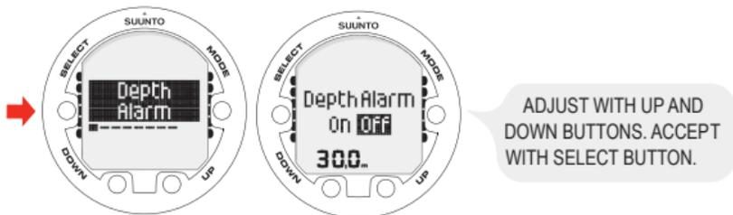
The depth alarm is factory-set to 30 m/100 ft, but you can adjust it according to your personal preference, or switch it off altogether. The depth range can be set from 3 m to 100 m/9 ft to 328 ft.
