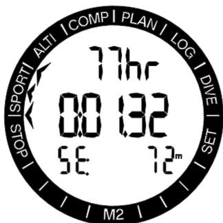
In SWIM mode and during surface exercise, the M2 displays the count of strokes or heart rate on the top row, the elapsed time on the middle row and the converted total distance on the bottom row.
