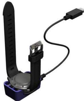
Communication between the M2 and the cradle is established via the contact on the case. Therefore, if the water contact or the spring contact of the cradle has surface dirt, this should be cleaned with a piece of cloth before use.
