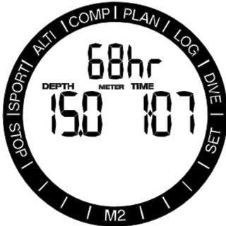
On the bottom row, the surface interval counter counts to 15 minutes. If no repetitive dive is done, the M2 reverts to the APNEA mode menu display.
