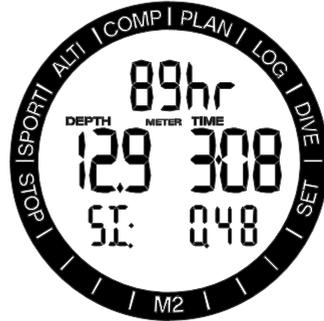
When the SIF is enabled, the no-dive symbol will be shown at the surface until this period has elapsed. An audible signal is given after this.
