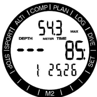
After a dive, the GAUGE mode surface display shows the dive time on the middle row. On the bottom row the stopwatch is running from the dive start or the last manual restart. On the top row the maximum depth of the dive is shown. After a 5-minute timeout the display changes to the GAUGE mode menu.
