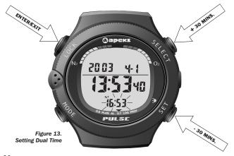
Dual Time shows the time in a different time zone, a handy feature when travelling. If Dual Time matches current time, it will not be displayed.
