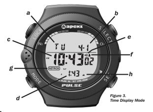
The Pulse's default mode is the Time Display Mode (figure 3). The computer always returns to the time display after making a dive or exiting from one of the other modes, such as Plan Mode or Log Mode. If there is no button activity for several minutes while in another mode, the computer will automatically exit back to the time display.
