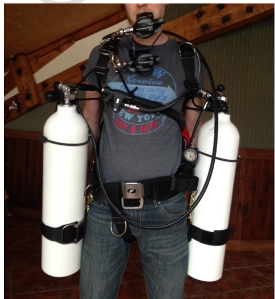
Pic. 13 Attaching the regulator – Right tank
