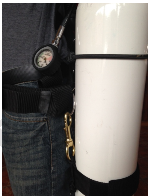
Pic. 10 Attaching tank - bottom
