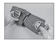
2. Unthread the waistband buckle. Connect the holster by feeding webbing through the rear holster loop (a), then the attachment loop (b) and finally the front holster loop (c). Slide the holster along webbing until its grommet holes (d) align with the selected grommet holes on the attachment (e) (Figs. 2 & 3).
